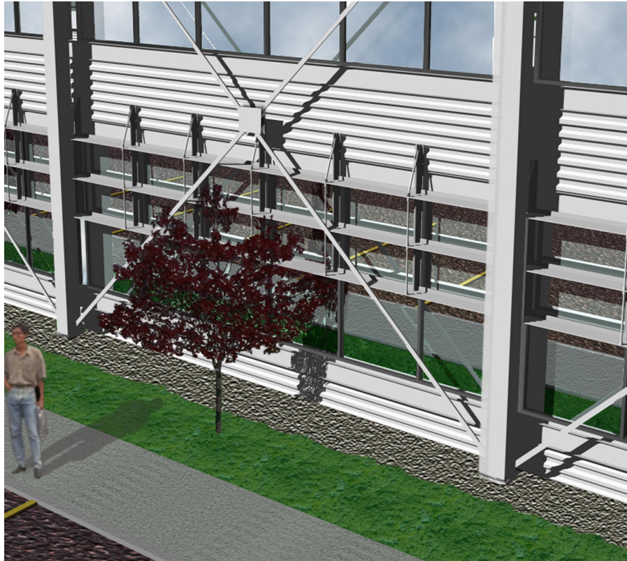
Figure 2. External view of 3-tier 1 ft. deep external shading devices proposed for Tech Office building
